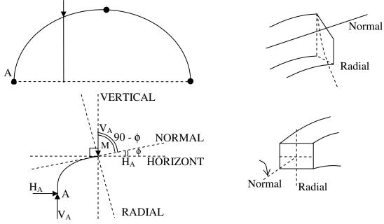
Total force acting along the normal is called normal thrust and total force acting along the radial direction is called radial shear. For the case shown in fig normal thrust
